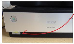
Make sure the scanner USB cord is plugged in to the computer you are using and that the scanner is turned on.
